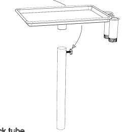
4: Insert neck tube (the thinner one) into the top of the base tube and use the knob to secure at desired height.
